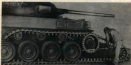
Figure 161—Removing Track by Turning Sprockets
