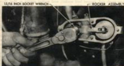
Figure 64—Loosening Rocker Adjusting Screw Lock Nut
