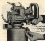
Figure 269—Cleaning Control Box Valve Plunger
