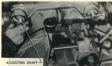
Figure 131—Steering Brake Shoe Adjustment
