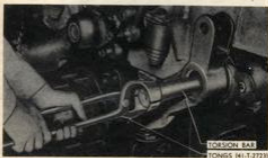
Figure 176—Removing Torsion Bar, Using Tongs 41-T-2723
