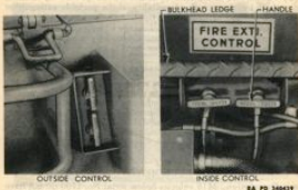
Figure 27—Fixed Fire Extinguisher Controls—M39
