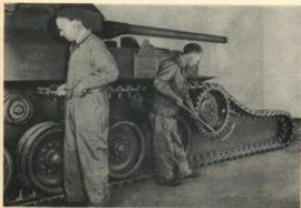
Figure 165—Installing Track Over Support Rollers
