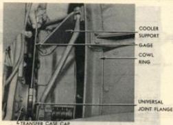
Figure 71—Checking Engine Alignment With Gage 41-G-13-300
