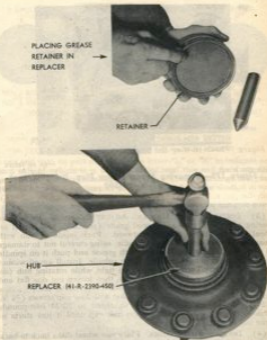
Figure 174—Installing Grease Retainer With Replacer 41-R-2390-450
