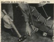
Figure 159—Starting Removal of Track Link Pin
