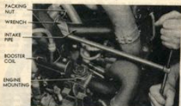
Figure 59—Removing Intake Pipe Packing Nut With Wrench 41-W-1537
