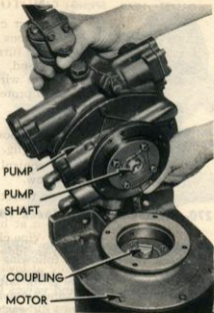
Figure 271—Installing Pump on Electric Motor
