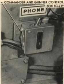
Figure 305—Commander's and Gunner's Control Box BC-739 Installed—M18
