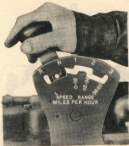
Figure 12—Operating Manual Shift Lever
