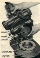
Figure 271—Installing Pump on Electric Motor
