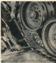
Figure 166—Installing Track Link Pin
