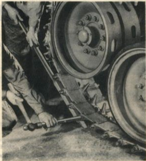
Figure 166—Installing Track Link Pin
