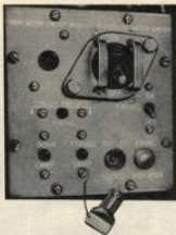
Figure 18—Turret Wiring Switch Box
