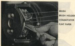
Figure 194—Cleaning the Generator Commutator
