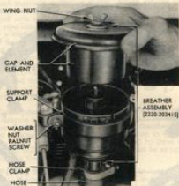
Figure 57—Removing Crankcase Breather Cap and Element
