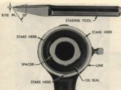
Figure 167—Oil Seal Staked in Link—Staking Tool Required
