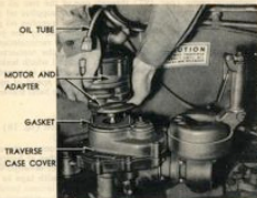
Figure 267—Removing Hydraulic Motor and Adapter
