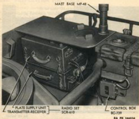
Figure 303—Radio Set SCR-610, Control Box BC-739 and Mast Base MP-48 Installed—M39
