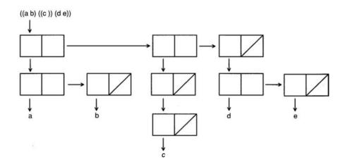
Figure **3.4:** Cons Cell Diagram of a Tree
