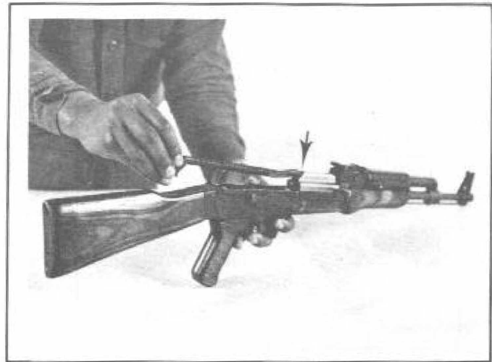
FIGURE 43. REPLACING DRIVING SPRING
