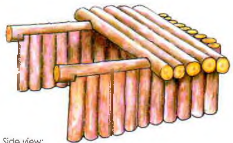
Side view: In order to improve stability the back wall should fit closely with the top edge of the roof. (The back wall can also have a cap log.)
