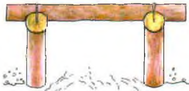
The cap logs are cut lengthways to fit the length of the walls and nailed to the top of them.
