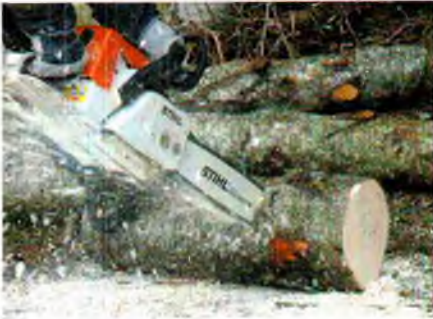
Notching the logs
