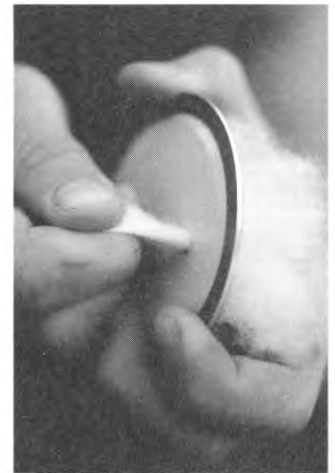
Making airport lids. Once cured and set up with a filter, these versatile lids can be used for most aseptic practices.
