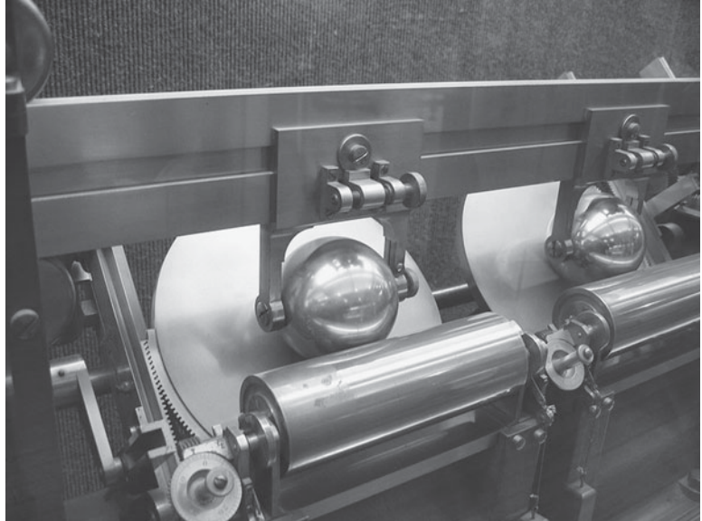
Fig. 3.11 The original integrator developed by Thomson.
