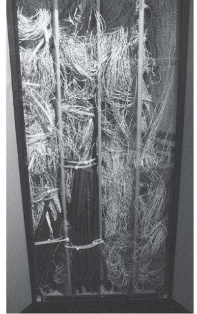
Fig. 5.20 For larger numbers of connected elements, crossovers can lead to the sort of rat's nest seen in the backwiring of a Cray computer of the 1970s. Photograph due to 'brewbooks' under creative commons license.
