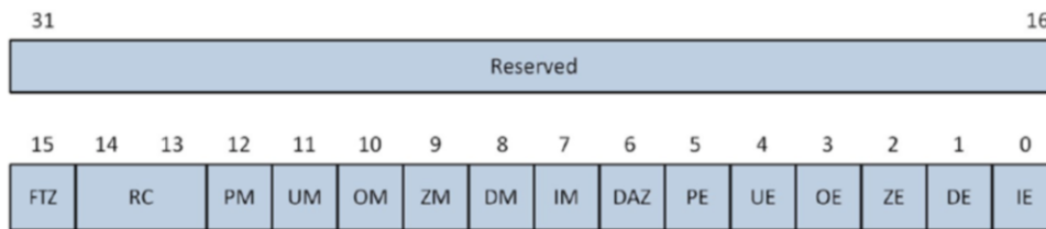
Figure 4-11. MXCSR control and status register
